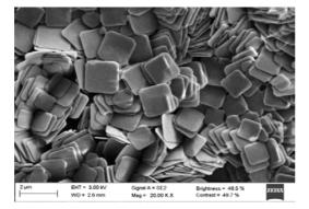
Here hybrid nanomaterials with properties derived from metallic NPs and MOFs were produced. The hybrid nanostructures were synthesized by growing ZIF-8 (Zeolitic Imidazolate Framework) around pre-stabilized NPs. UV-Vis spectroscopy, X-ray diffraction, dynamic laser-light scattering (DLS), SEM and TEM were performed in order to characterize the physicochemical properties and the morphology of the composites.
